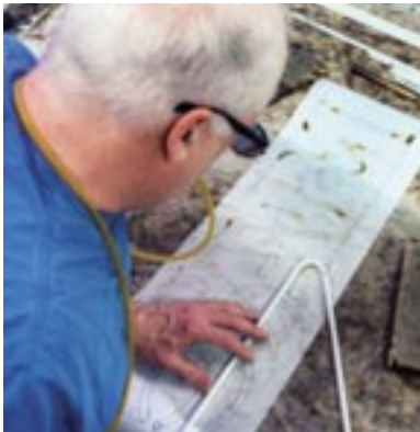
Left: “Neon Mike” Lacroix bending glass tubes in his workshop in Grand Rapids, MI. Right: Shaping the neon tubes.
