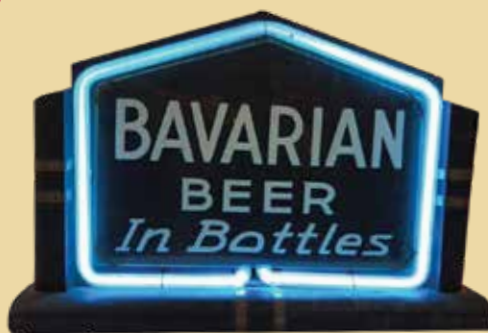
Bavarian (Bavarian Brewing Co.) back bar neon sign, c. early 1940s by The Lackner Company, Cincinnati, OH. Glass, gas-discharge tube around reverse-etched/painted ad panel in painted metal cabinet with chrome-plated trim, collection of Matt Russell.
