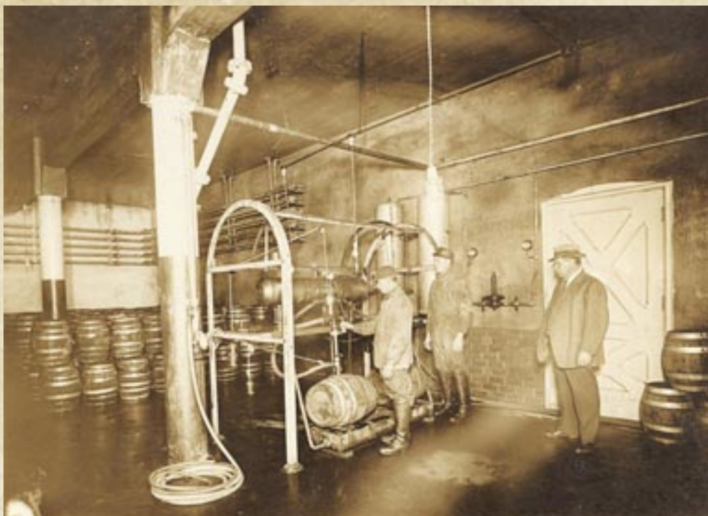
Keg filling machine at Little Rock Brewing & Ice Co., c. early 1900s. Courtesy of Butler Center for Arkansas Studies.
