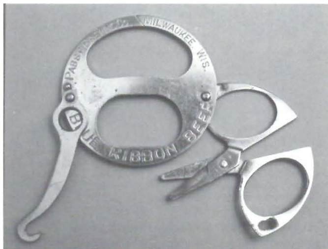
Fig.1: And you thought openers were just church keys and the occasional corkscrew? This is JFO M-78-1, from Pabst, a 1914 patent by Hesuah. Button hook, scissors, cigar trimmer, crown opener and key ring, all in one!
