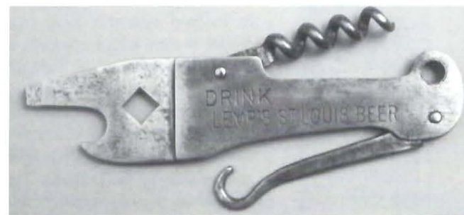
Fig 10: B-45-1, from Lemp, St. Louis/ C.H. Reilly Dist. Salt Lake City. The "I" denotes copy on reverse side. This stamped steel opener has a corkscrew, button hook, Autolite key (the diamond-shaped hole, for turning on old acetylene car headlights), a crown lifter and hole for key chain.
