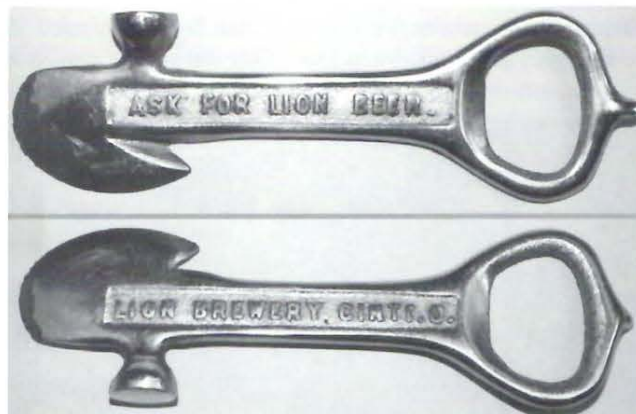
Fig 8 & 9: Another multi-purpose cast iron opener, with both sides shown. This cigar box opener (D-8-2, from Cincinnati's Lion Brewery) has both a crown lifter AND the small hook to remove the Baltimore Loop Seal closure, another William Painter patent. The tapered end slips under the box lid, and the hammer reseats the brad that held the wooden cigar box closed
