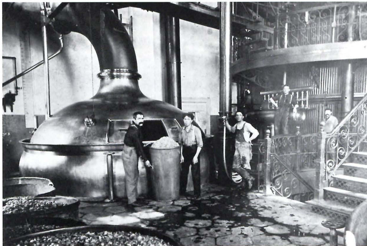
Hops are about to be added to a kettle from baskets holding weighted amounts. System remained unchanged until use of pelletized hops permitted automatic hop addition beginning in the late '60s. Minnesota Historical Society.
