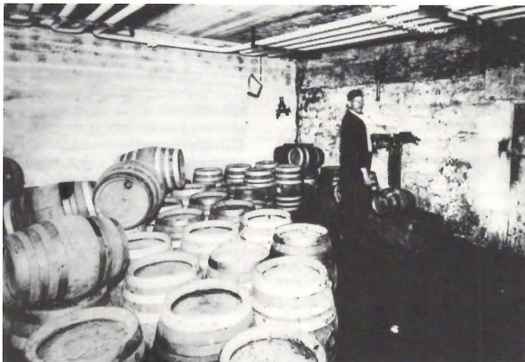
Above: Racking cellar is cramped but contains good cooperage. Coils on ceiling show frost condensation on pipes containing circulating expanding ammonia. Below: Bottle shop is equipped with straight-line filler and simple basket pasteurizing tank. Boy in background standing in front of beer pump seems smaller than those usually seen in brewery group photos. Wall calendar shows September 1908. Original photos belong to Norman Yogerst.
