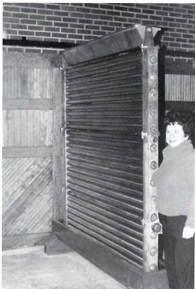
Helen Haydock with a wort cooler. Beer went over the out side and the coolant was on the inside.
