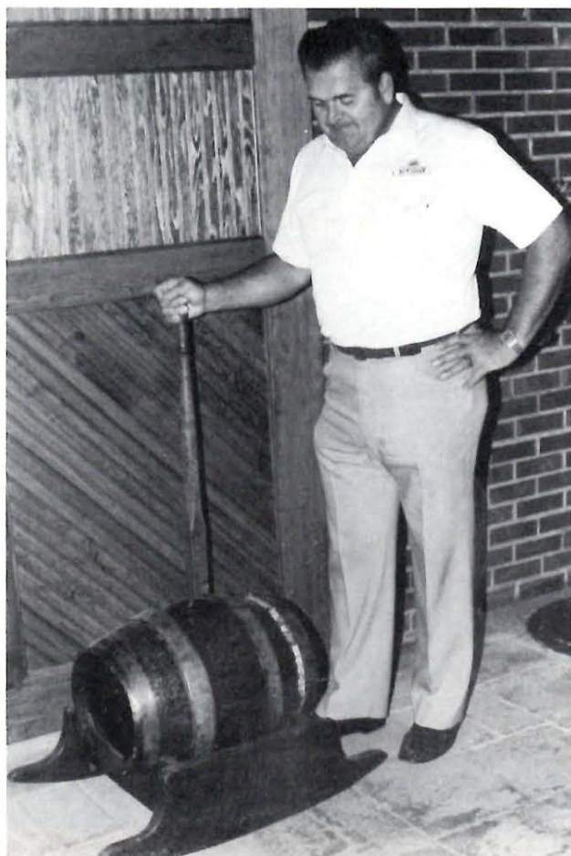
Herb Haydock with a tool called a keg rocker. Beer and Hops were put into the keg and the keg was closed up. Then the keg was rocked This is called cold hopping.
