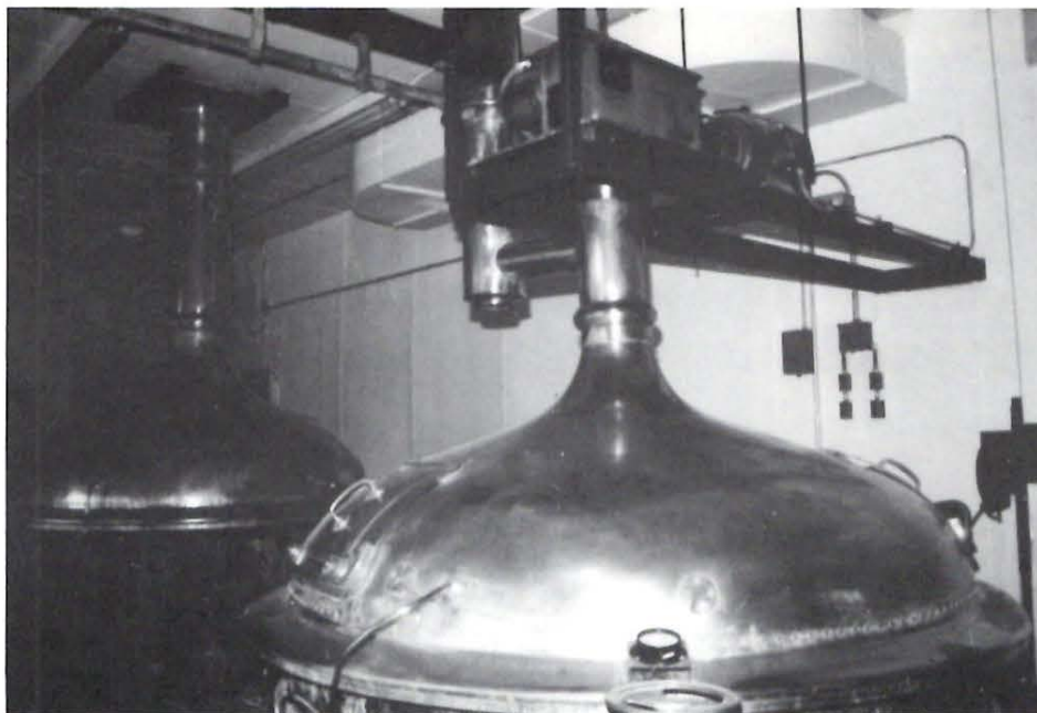
In Capital's brewhouse, the mash tun is at left and the the brewkettle in the foreground. The copper vessels are of a size suitable to a small local brewery. The micro-brewers typically use small stainless steel vessels.
