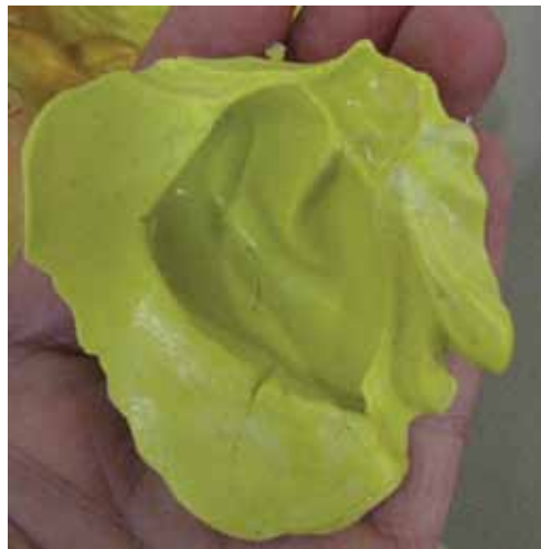
Flexible mold of the piece to be cast with the resin.
