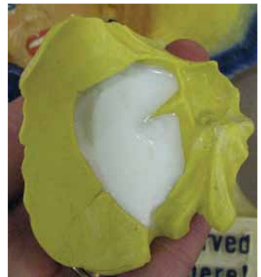
The resin mix will turn opaque white in about 5-10 minutes, when hardened and ready to remove from the mold.
